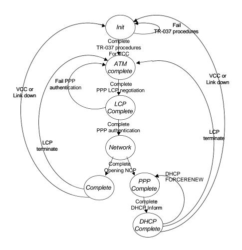
Figure B.1 Generic PPP state transition diagram
