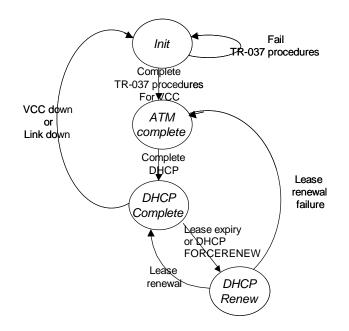
Figure B.2 Generic Ethernet state transition diagram
