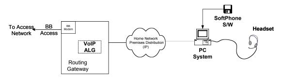
In this scenario, the VoIP functionality is added to the PC via VoIP Software (3rd party or part of the PC operating system) and it is this VoIP software, embedded within the PC, which processes the VoIP call. A speaker and microphone are also required for VoIP operation. These may be either internal to the PC or added as external peripherals, e.g., a headset. The RG may have no VoIP awareness/capabilities or have a VoIP application layer gateway (ALG).
