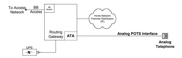
In the example given in section 3.1.1, both the RG and the Standalone ATA are plugged into an uninterruptible power source (UPS). In this example, only the RG will make use of a UPS (external or internal batteries) and the ATA will draw its power requirement during a power outage directly from the RG. In this scenario, , the RG and hence ATA will not cease to function in the event of a commercial power
