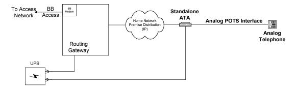
In the above example, both the RG and the Standalone ATA are plugged into a UPS. In this scenario, as both the RG and the ATA are plugged into a UPS, neither the RG nor the ATA would cease to function in the event of a commercial power failure, thereby ensuring a continuous VoIP service. In cases where a UPS is employed to ensure continuous voice service no standard POTS is required.
