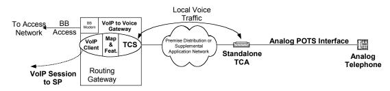
The RG with Voice to VoIP Gateway Capability allows the RG to act as the VoIP endpoint in the customer premises, and support multiple thin-client voice endpoints inside the premises.
