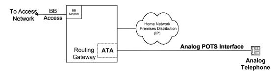
This configuration is similar to the configuration of a Standalone ATA presented in section 2.1. In this configuration, the ATA functionality is physically located or embedded within the RG. The ATA processes the VoIP call and presents it to the analog telephone via the standard analog telephone interface located within the RG. In this configuration the RG is VoIP aware. The RG with embedded ATA functionality may have more than one physical port for supporting multiple derived lines.
